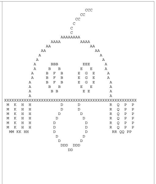
which defines the ''strokes' that the machine is to make. Each stroke is labeled by a different capital letter. The machine repeatedly goes to one end of a stroke, executes a pendown, moves to the other end of the stroke, executes a penup, and then moves to one end of the next stroke, or if done with all strokes, moves to its starting position. The machine never omits the penup at the end of a stroke, even if the next stroke begins in an adjacent square.
